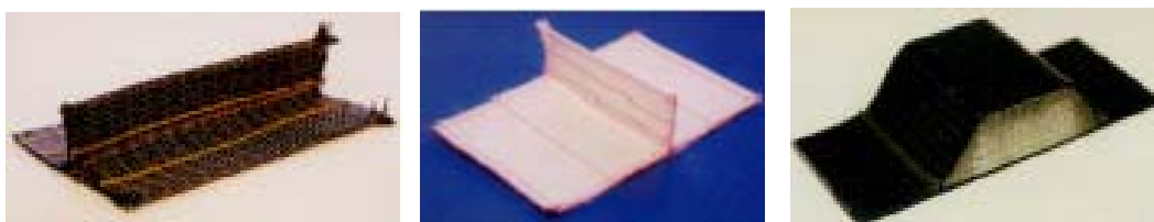
Fig. 5 3-dimensional technical textile products from glass and carbon fibres
