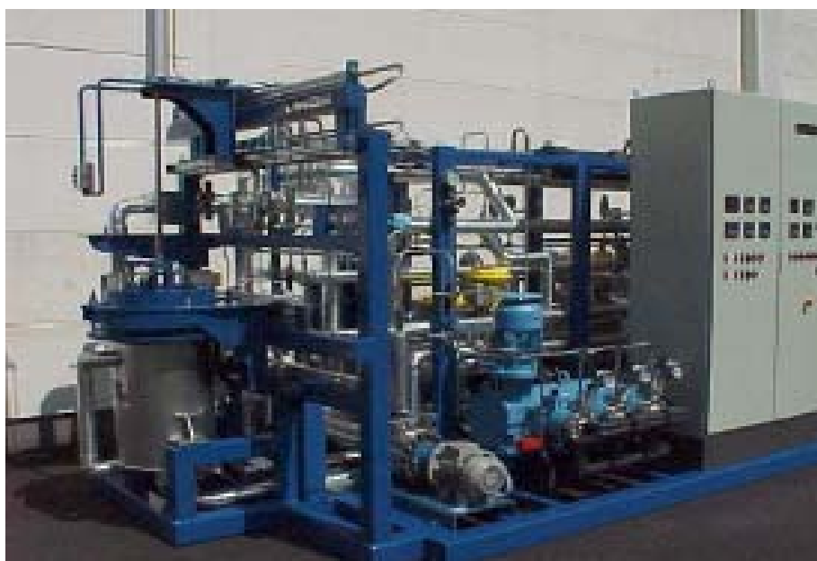
Fig. 12: pilot system for textile dyeing with overcritical CO 2 (source: DTNW Krefeld)
